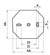
materiál - úprava (barva) / material - surface finish (colour) : nerez 1.4301-broušená nerez stainless steel 1.4301-brushed stainless steel
