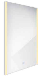
LED mirror 500 x 700 With touch sensor. Possibility of setting the color temperature 2700K - 6000K. Output 21W. Aluminium frame.
