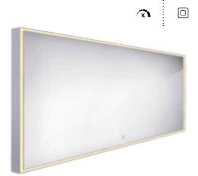
LED mirror 1400 x 700 With touch sensor. Possibility of setting the color temperature 2700K - 6000K. Output 60W. Aluminium frame.
